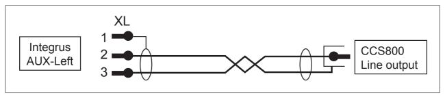
Figure 3.2 Wiring of the cinch to XLR connecting cable
